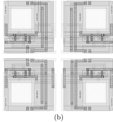
Figure 2: Circuit architecture of the designed CMOS image sensor(a) and four types of the pixel circuit layouts(b).
